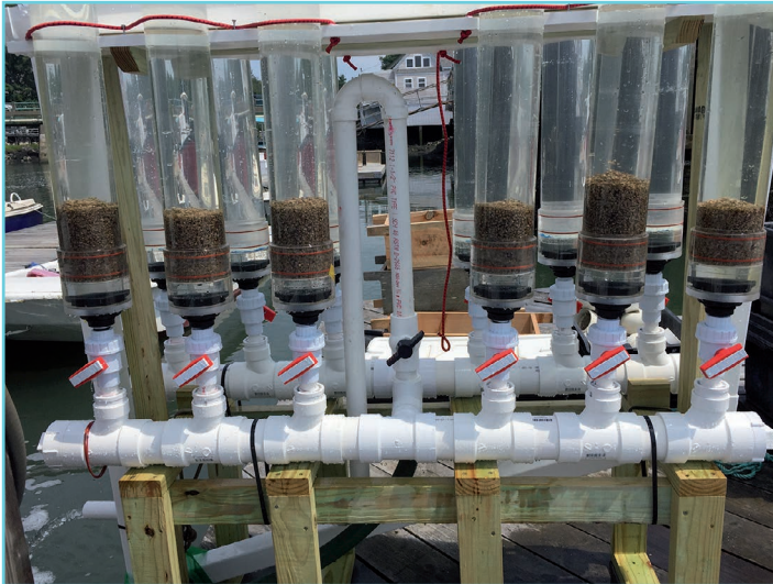
Figure 1.10 Small-scale tubular upweller system for use with juvenile oyster seed. Courtesy of Chris Davis.
