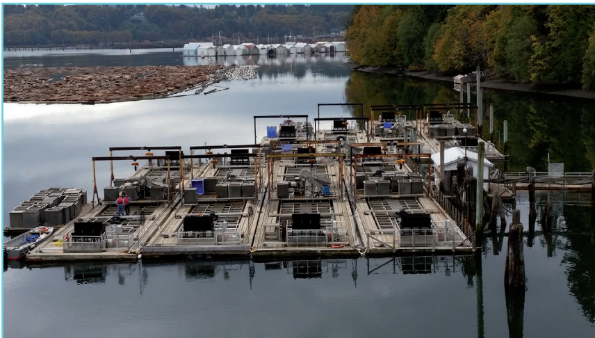
Figure 1.9 A large multi-bin upwelling system in Washington State. Water flow in large systems are best driven by slow turning paddle wheels. Courtesy of Taylor Shellfish Company.
